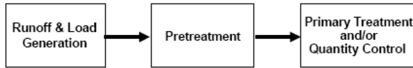
FIGURE 4-34 Generalized Stormwater Treatment Train
